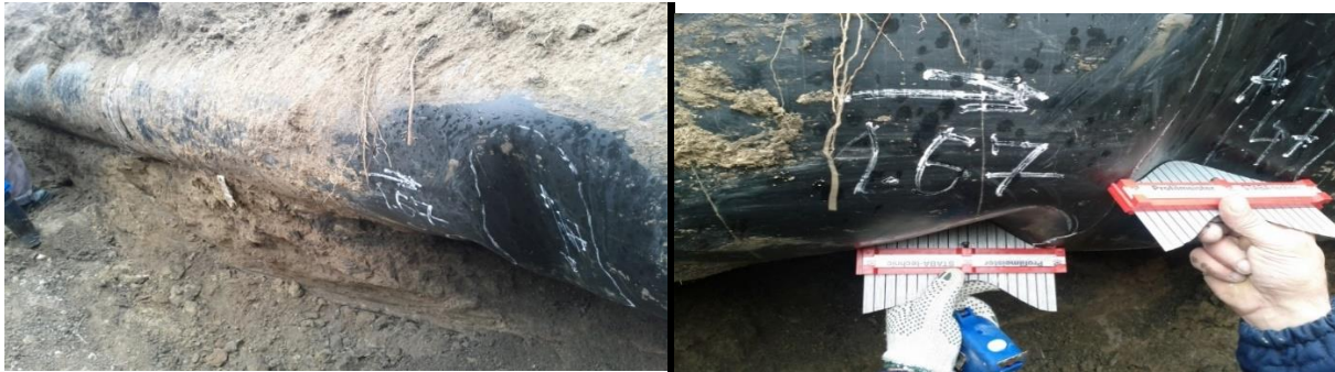
Image 5 - 2-plane deformation (mechanical stress) – removed
