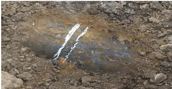
Image 1 - Generalized pitting located in the upper part of the pipe - totally destroyed external insulation (temporary repair)
