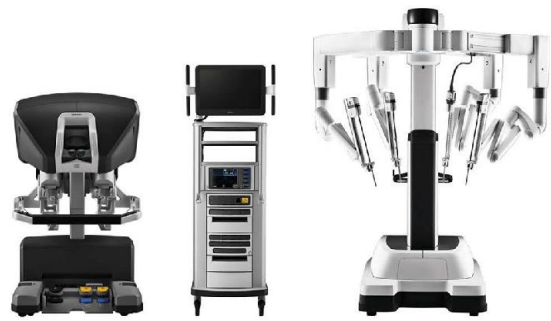
Figure 1. da Vinci surgical system. Source: Intuitive Surgical
